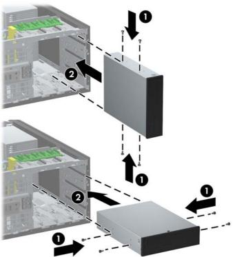
Figure 5-23 Installing a 5.25-Inch Drive in a Minitower (top) and Desktop (bottom)
